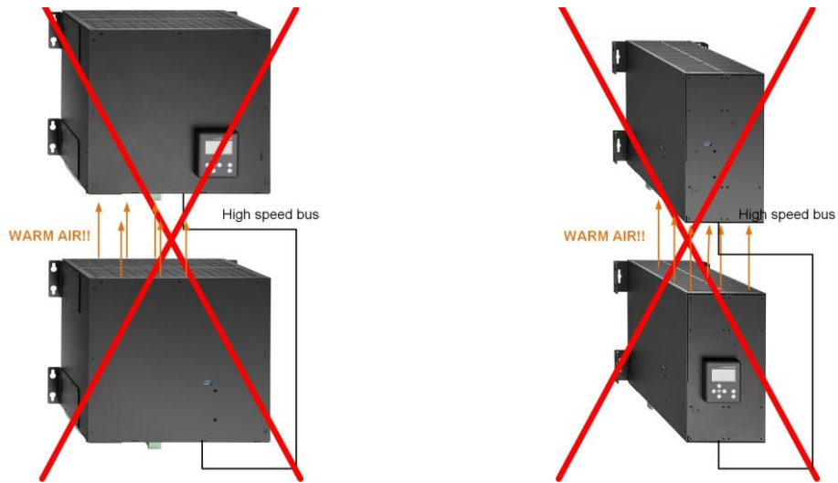
Figure 11 Wrong ways to install DPP
